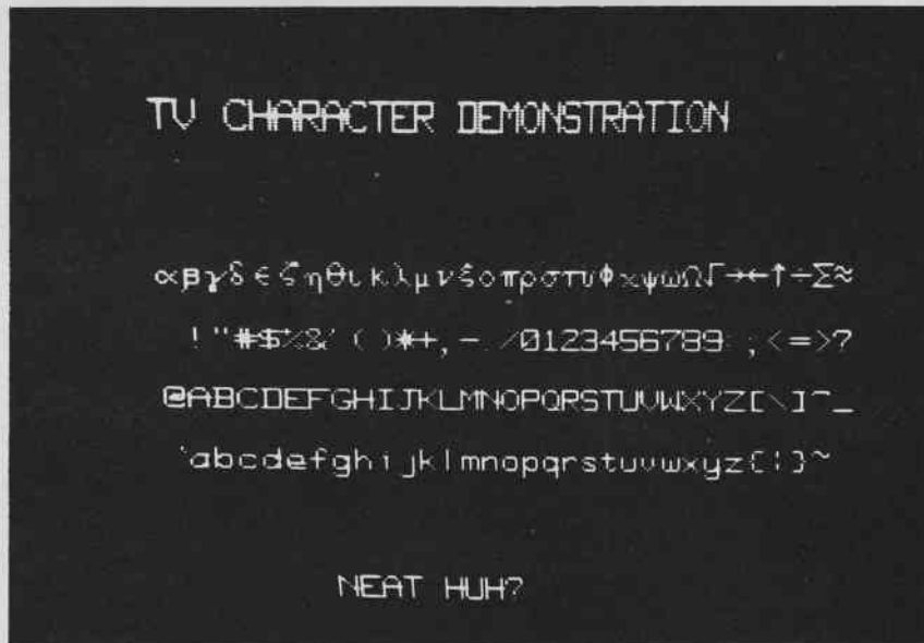
Photo 1: A test demonstration of Dr Suding's TV readout, shown in schematic form as figures 1 and 2. The test pattern consists of the four lines in the center which cycle through the possible binary combinations of characters. The differences in line width between the top line and the other lines are caused by non-linearities in the monitor used for this photograph.
