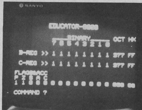
Photo 1: In this example, Educator-8080 is shown before (left) and after (right) the execution of an XRA A instruction. The effect of this instruction is of course to clear the accumulator A, as is shown at the right.
