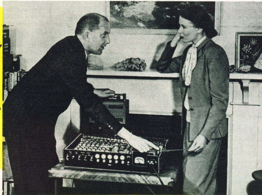
E. C. Berkeley explains how Simon gets instructions from a piece of punched tape.
